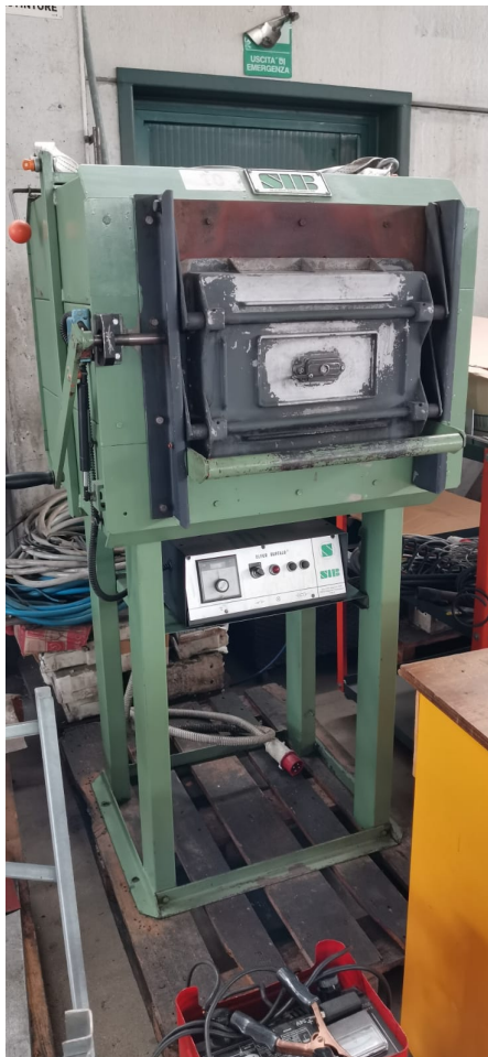
Hardening and tempering furnace 1100 degrees
