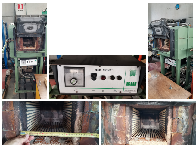
Hardening and tempering furnace 1100 degrees
